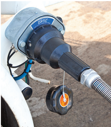
One Connection for Overfill Prevention and Earthing
