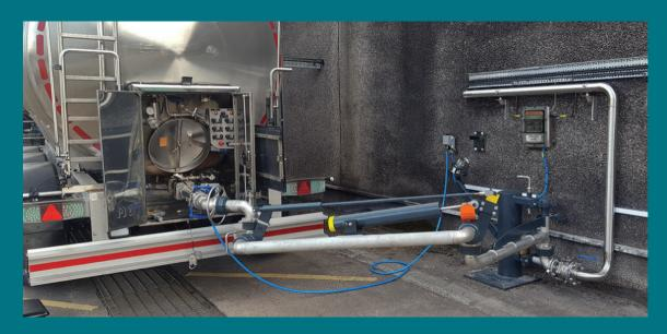
Scully overfill prevention sensors are mounted in each tank truck compartment through an aperture in the man lid assembly and are set at a predetermined safe level.
