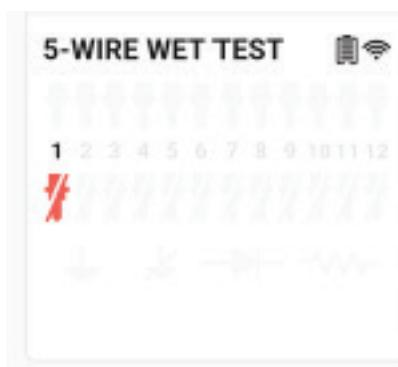
5-wire sensor circuit faults can take on several forms. One option is the interruption of the diagnostic line. If the MTT is running the wet-test and the diagnostic line is interrupted, (but all other connections are working) the MTT will not indicate a fault on the screen. This is unique to a single sensor configuration.
