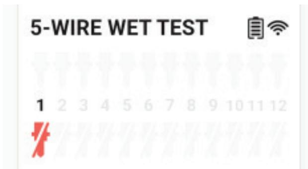
A similar scenario would be the failure of the yellow wire (pin4) circuit. In this case, the MTT display will only show a single red sensor after initial detection or during the wet-test. Hence, if you see either of these two displays, you can determine which pulse circuit (pin 4 or pin 6) is most likely at fault.
